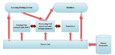
Fig. 2: Sensor Node Architecture [5]
