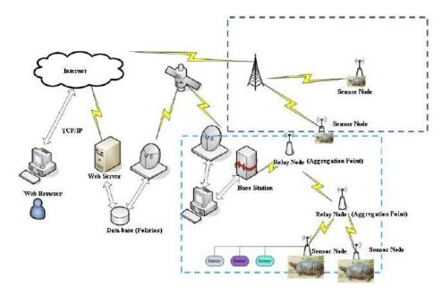
Fig. Error! No text of specified style in document.: A simple wireless sensor network
